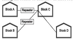
For layout 2, since the distance between Blocks A and C is large so a repeater would ideally be placed in between this path.
